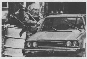
AN OPERATION: ALBUQUERQUE participant uses the PAN Disrupter to disable a bomb on the front seat of a parked car.
